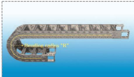
New Sabin Chain's turning radius is larger than that of its inserted cables. To find a suitable bending radius for your application, as a rule you should multiply the outside diameter of your largest inserted cable by 8-10 times.
