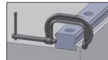
Fig1.8.13 Mounting the master Linear Guide rail
