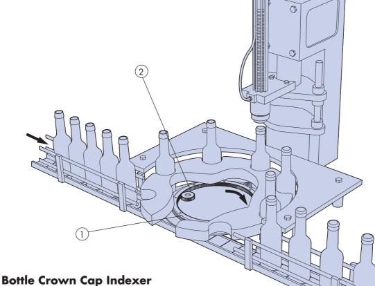
Bottle turn table is mounted on a HepcoMotion single edge ring slide
